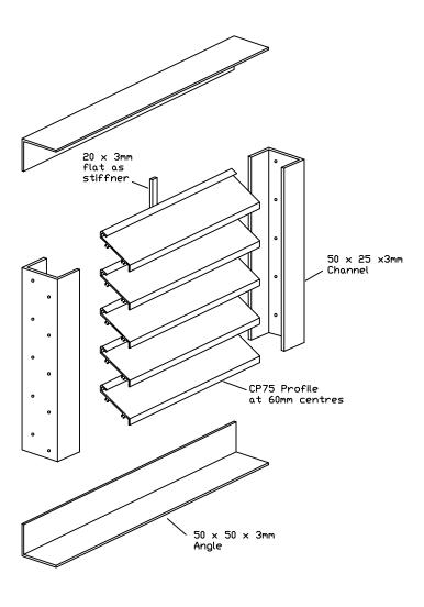
NDTES: 1. Need 20  $\times$  3mm stiffner every 1000mm 2. Need 50  $\times$  50  $\times$  3mm Angle top and bottom if have stiffner
